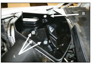
**8.** A) Determine the stud size of your particular vehicle, and secure the CAB using the appropriate washers and nuts. Vehicles with SAE studs will use the 1/4" x 20 Flanged Nuts (#10) and three Fender washers (#11). Vehicles with Metric studs will use the 6mm Flanged Nuts (#9) and three Flat Washers (#11). **B**) Re install the Factory 8mm bolt thru the CAB and into it's original location.
