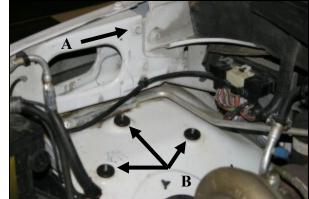
**6. A)** Remove the Factory 8mm fender bolt and set aside, it will be reused later in step 8. B) Place the 1/4" I.D. Grommets (#12) over each of the three studs on the inner fender.
