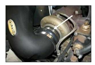
7. A) Install the CAB and Tube assembly onto the turbo inlet first, then rotate the assembly downward onto the inner fender studs. B) Secure the Silicone reducer to the turbo inlet using the # 64 Clamp (#13). C) Fully tighten the three 1/4" Button Head Bolts from step 4. Apply the Airaid Bubble Decal onto the Intake Tube as shown.
