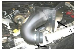
5. A) Install the aluminum Heat Shield (#4) onto the CAB using the four 1/4" Button head Bolts (#7) and the Flat washers (#8). Remove the protective film from Heat Shield. B) Install the silicone reducer (#5) on to the Airaid Intake Tube (#2) using the #80 (#14) Hose Clamp.
