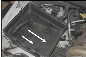
3. Locate the fender air scoop inside of the factory air box and remove it by pulling outward. The remaining factory airbox half can now be removed by simply pulling upward and off of the mounting studs on the
